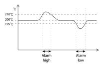
Above drawing shows two alarming cases when you set-up alarming Max. Limit with 10  $^{\circ}$ C, alarming Min. Limit with 5  $^{\circ}$ C. Alarm sounds during operation of equipment.
