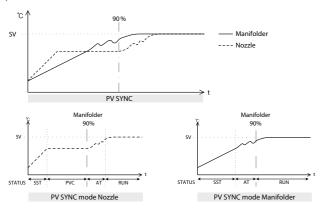
As per two drawings above, at the time of Completion Of Nozzle's Soft Start, it controls nozzle and manifold separately. Nozzle will maintain the temperature of Soft Start until manifold gets heat 90% of SV Temperature. And when manifold gets over 90% heat of SV, Nozzle Gets Heat to reach SV at about same time as MANIFOLD. You can change preset value according to Change of set-up value ③(page 27).
