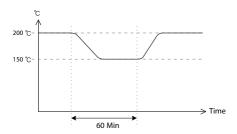
Above drawing shows operation with 150  $^{\circ}$ C STANDBY Temperature and 60 min. STANDBY Time.
