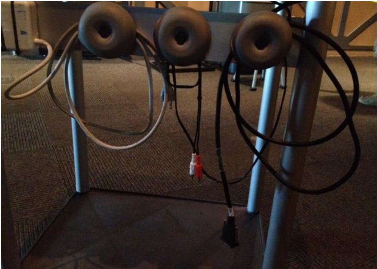
Figure 2 showing laptop cords and plugs. From left, you'll see the power plug, then audio plugs and DVI plug.
