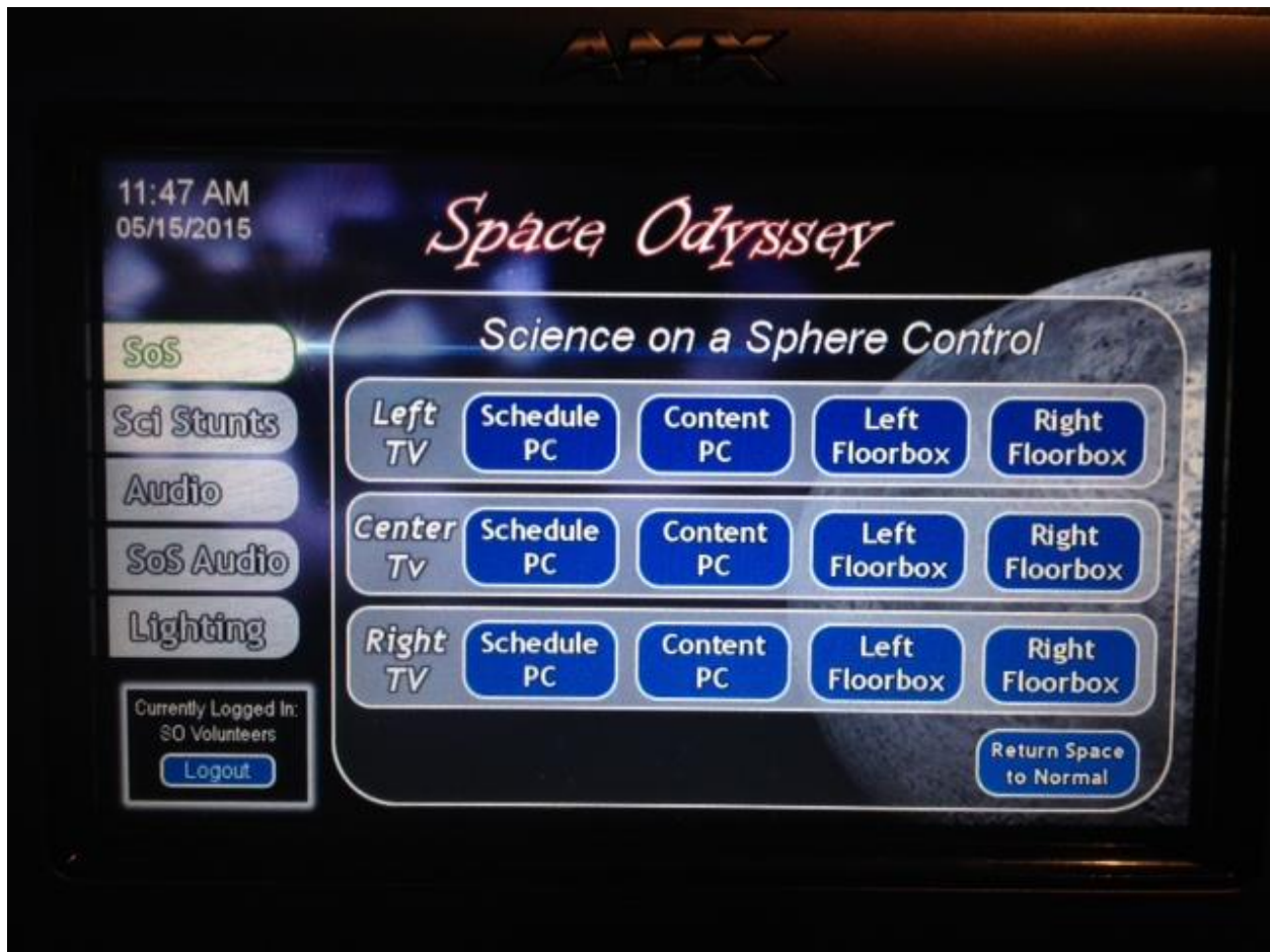
Figure 8 shows the “SOS” menu which allows you to send the image from a laptop/iPad to any of the three screens around the SOS. Note the “Return Space to Normal” button at the bottom right which, when tapped, will let you reset the space once you’re done using it.
