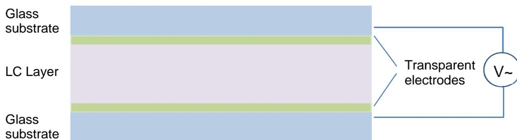
Figure 1. Transverse view of the VSP: Liquid crystal layer between two glass substrates with transparent electrode. Optical axis director can be tilted with the help of an applied bias  $V$ .
