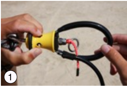
1 Push the yellow Ejector upwards and away from you to open the system.
