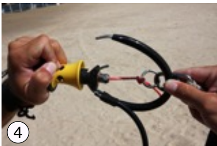
4 To re-assemble the system hold the Chickenloop in one hand and push up the yellow Ejector with the other hand.
