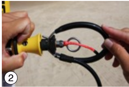
2 This releases the Safety-pin.
