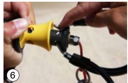
6 Now guide the metal loop and the Safety-pin back into their designated grooves.
