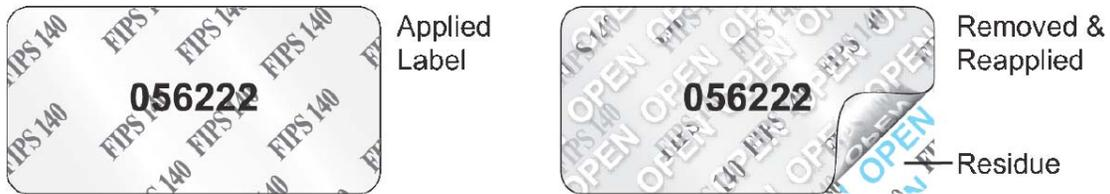
Each TEL has a unique serial number to prevent replacement with similar label. To protect the device from tampering, TELs should be applied by the Crypto Officer as pictured below:
