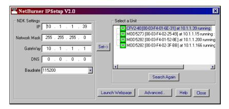
Click the "Search Again" button to locate your unit in the "Select a Unit" pane. If your Paranoia3 unit does not appear, verify the power and link LED's on your MNGT connection on the front panel are illuminated; if not, correct any cabling errors. Note that IPSetup uses a UDP broadcast protocol similar to BOOTP and will **not** operate through a router.
