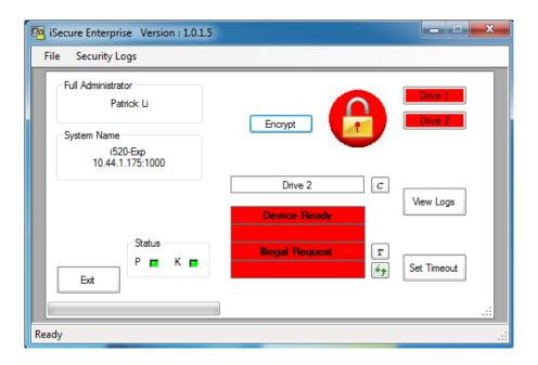
The tape drives must be either unloaded or at BOT for the keys to be downloaded. If you get the message as shown below use the system to unload or rewind the tapes to BOT and then try again to connect to the unit.
