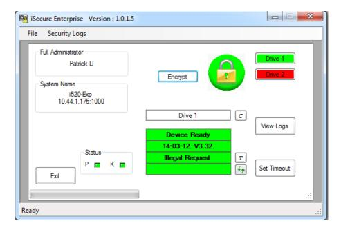
For a multiple drive connections first select the correct drive using the Drive number button (if only one drive is connected this will not be applicable) then select the Encrypt button. As long as the tape is either at BOT or unloaded the display background will go green and this drive is secure as shown below.
