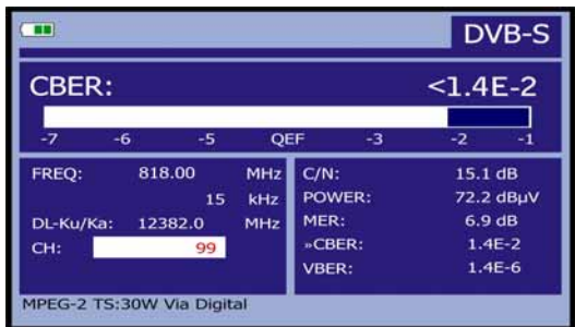
Figure 35.- DVB-S (QPSK) signals CBER measurement screen.
