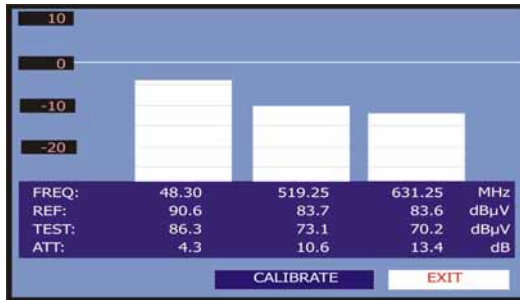
Figure 13.- Attenuation Test. Terrestrial band.
