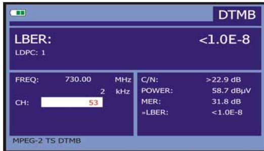
Figure 34.- DTMB signals LBER measurement screen.
