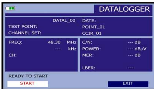
Figure 14.- Datalogger screen for Attenuation test frequencies.
