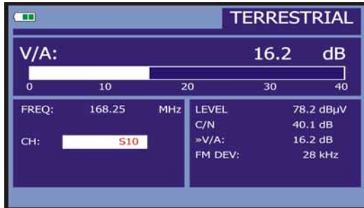
Figure 23.- Measurement of the video/audio ratio.
