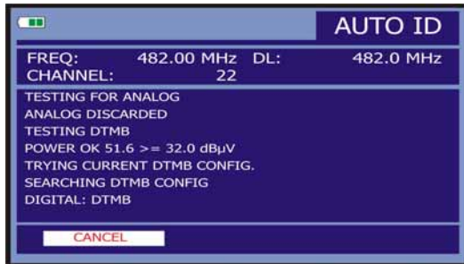
Figure 9.- Signal automatic identification screen. AUTO ID.
