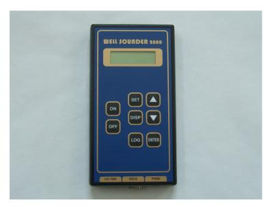
POWER ON TO DEPTH DISPLAY: Press the ON button located on the front panel of the control unit. The probe will pulsate and the LCD screen will display the default operating screen. The depth is displayed on the top line. Press the arrow buttons to view additional information displayed on line two such as the battery voltage, the optional flow meter, or the temperature sensor.
