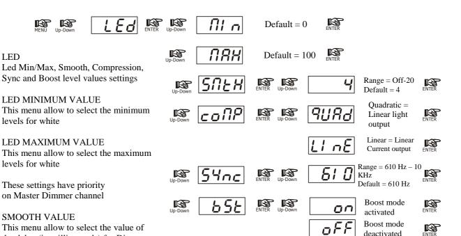
With BOOST active, the LED'S current is set to Max value. (30% more gain compared to BOOST Off)
