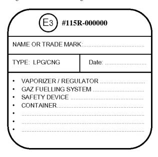
The above plate, with approval mark and some technical information on the retrofit system, has to be fixed permanently on the body of the vehicle.
