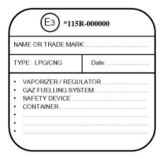
The above plate, with approval mark and some technical information on the retrofit system, has to be fixed permanently on the body of the vehicle.
