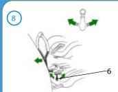
Adjust the front brace outwards with the ratchet (6). Continue tightening until the brace is pressed well into the backrest of the car seat.
