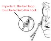
The floor support (12) must go through the belt loop (14). The belt loop must also be led into the hook on the floor support.
