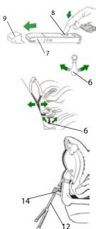
Remove the plastic caps (9) from the ISOfix connectors (7) by pressing down the ISOfix release button (8).
