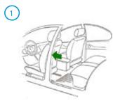
If your iZi Kid ISOfix is installed in the back seat, push the front seat as far forward as possible.
