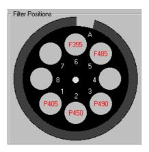
There are also two optional filter wheels: filter wheel B and filter wheel B2. Filter wheel B(left side figure) has four positions for the most common size of commercial filters i.e. "round one inch". Filter wheel B2 (right-hand figure) has 8 positions for filters with a diameter of 15 mm. Both wheels are supplied empty but with locking rings.
