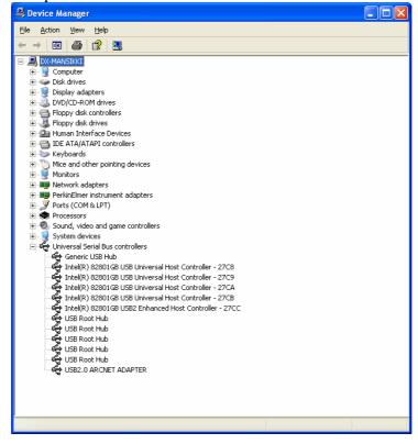
Right-click to see the properties of the adapter. Check the device status.
