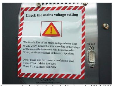
Its purpose is to alert you to the fact that the fuse holder is set for 220-240 V.
