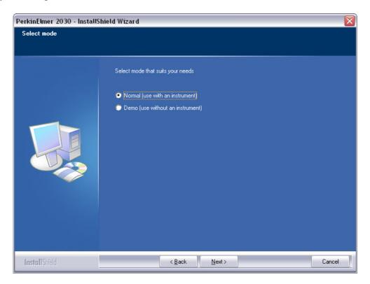
Click **Next** if your PC is connected to the instrument. With no instrument, the workstation can be run in demo mode and the software itself simulates the instrument. In that case select **Demo** and click **Next**.
