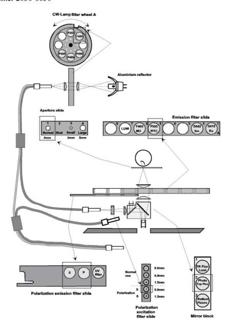
Light is produced by the same tungsten-halogen continuous wavelength lamp used for normal fluorometry and photometry. In fluorescence polarization, the excitation energy control is only by means of the constant voltage mode. The lamp is run at full power, with no voltage adjustment.
