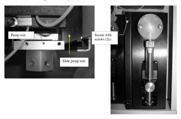
Connect the tubes (2x) to the pump unit as indicated in the pictures.
