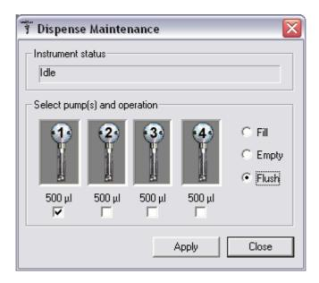
The setup dialogue presents you with a graphical representation of the number of pumps (1 - 4) available when performing an operation. You can select the pump(s) that are going to perform the operation by checking boxes under the respective pump pictures. The operation to be
