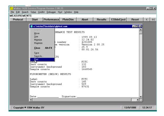
Check that the results are within the limits shown on the next page. Note that not all instruments have all the options and the different models have different limits.
