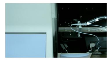
Secure the dispenser with the thumb screws (2x) (see the figure below).
