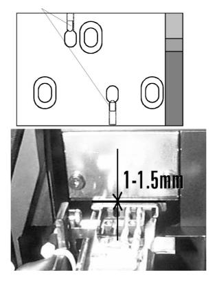
When the height is O.K, tighten the three screws.
