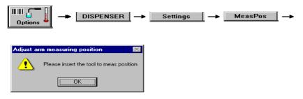
Insert the adjustment tool and click OK, then run the arm to the measurement position by clicking:
