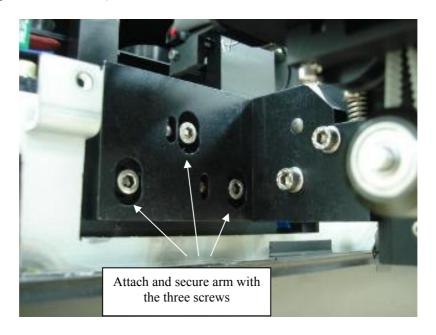
To adjust the height of the robotic arm - locate the arm to a couple of millimeters away from PerkinElmer 2030 and adjust the screws for the guide pins so that the height between PerkinElmer 2030 and the arm is 1-1.5 mm. Push the arm completely into the instrument and check that it moves freely without touching the measurement head on the way in.
