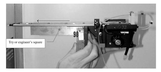
If they are not perpendicular, loosen (2x) and adjust (1x) the screws on the base (see the figure below). Turning it clockwise will adjust the robotic arm downwards while turning it anti-clockwise will adjust the robotic arm upwards.
