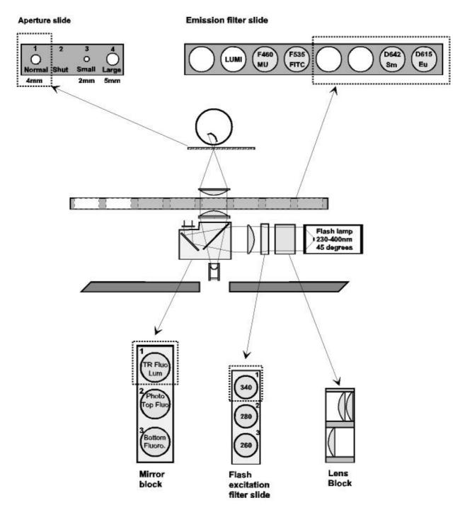
This configuration is used for both types of time-resolved fluorescence measurements i.e. DELFIA®, involving dissociation and enhancement, and LANCE homogeneous assays. For enhanced performance with LANCE it is possible to install an optional red-sensitive detection unit (PMT).
