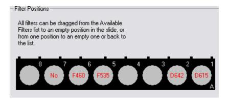
Emission filter slide A can be replaced with another one which has no predefined filters, so you can choose which filters you want to load. There are eight positions, the same as in filter type A. The size is "round one inch".
