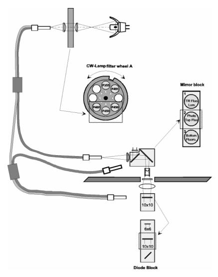
For absorbance measurements the same excitation system is used as for prompt fluorescence. The wavelength of the light can be in the range 320 -1000 nm.
