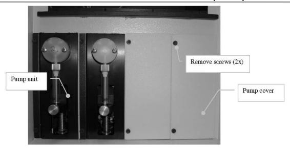
To install the pump unit, simply slide the pump unit into position (as indicated in the picture below) before securing it to the dispenser unit with screws (2x).
