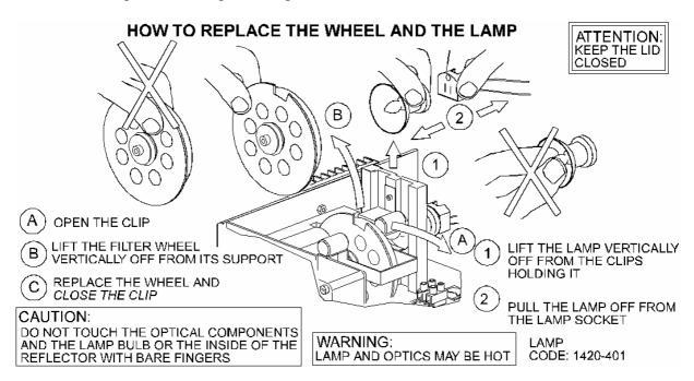
When you have replaced the lamp, close the cover and switch power on.
