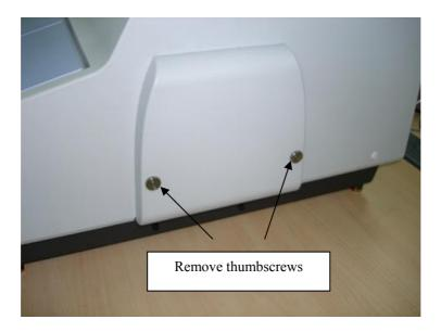
Remove the cover by unfastening the three side screws and the pressing on the two catches on the front end of the instrument (see fig below).
