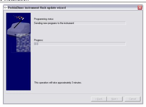
Warning! Do not interrupt this procedure by switching off the PC or the instrument. Wait until the update is completed because an interrupt can cause permanent damage on the microcontroller boards and the only way to recover from this is to replace the boards!
