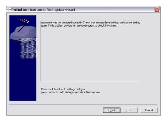
In this case the instrument was not switched on so the connection could not be established. Check connections and power and click the **Back** button when everything is OK.
