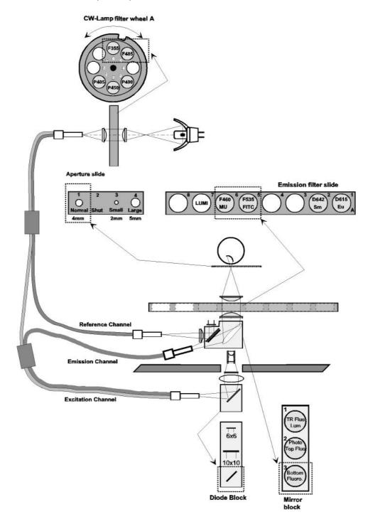
In the case of bottom counting of prompt fluorescence samples, excitation light is directed through a light guide underneath the plate. Emission light from the bottom of the sample goes back along the same light guide to the optical block where the emission filter is and from there to the PMT. Bottom counting allows measurements to be made for samples in which cells are at the bottom of the wells or there are lids on wells.
