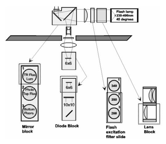
For UV absorbance measurements the same excitation system is used as for time-resolved fluorescence. The wavelength of the light can be in the range 230 -320 nm.
