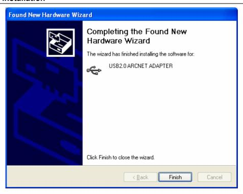
Complete the wizard by clicking 'Finish'. The installation of the USB22 ARCNET adapter is now ready.
