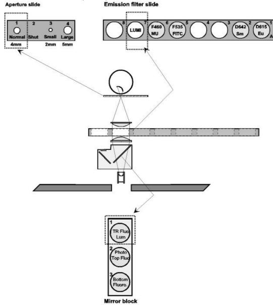
Measurement of glow, flash and dual-type luminescence is possible with PerkinElmer 2030. In luminometry there is no external excitation but the light is produced in the sample and then passes through a lens and an empty position in the emission filter slide to the photomultiplier. Although one filter position in the standard slide (A) is empty and is intended for luminescence measurements, any of the filters can be specified to be used with a luminescent sample.
