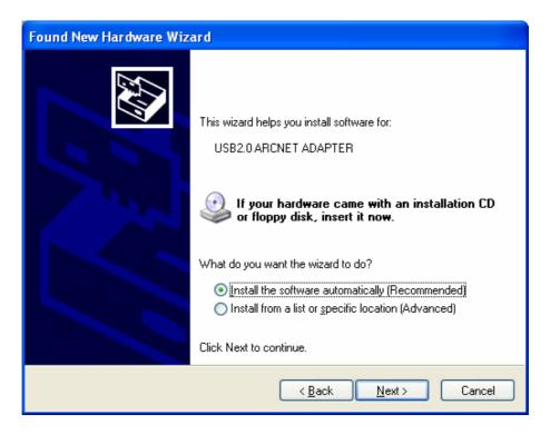
The USB ARCNET adapter is found and software for it will be installed. Select 'Install the software automatically' and click 'Next>'.
