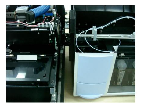
Connect the two connectors (Opto and Motor) for the robotic arm to the main instrument.
