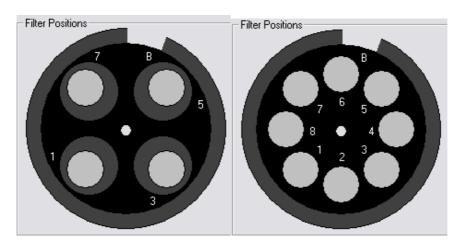
The system recognizes automatically if the type of wheel is A or B. However, if a B2 wheel is used instead of the default type B you need to inform the system through the workstation software. This is done by selecting "Use CW-lamp filter wheel B with 8 slots" in Tools/Options/General:
