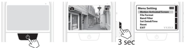
Press the **Power button** to go to the preview screen, at the preview screen, hold the **Up or Down button** for 3 seconds, and you will go to the menu setting screen.
