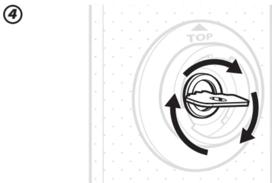
4. Use the Tightening Tool included to tighten the PeepHole barrel.
