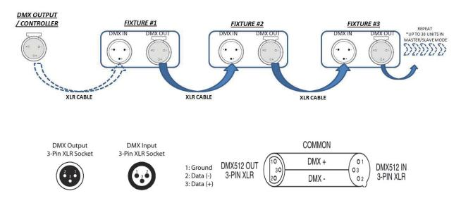
For installations where the DMX cable has to run a long distance, or is in an electrically noisy environment, it is recommended to use a DMX terminator. This helps in preventing corruption of the digital control signal by electrical noise. The DMX terminator is simply an XLR plug with a 120  $\Omega$  resistor connected between pins 2 and 3,which is then plugged into the output XLR socket of the last fixture in the chain. Please see illustrations below.
