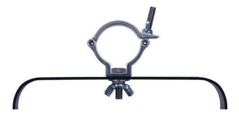
Regardless of the rigging option you choose for your MICROH PLASMAWAVE, always be sure to secure your fixture with a safety cable. The fixture provides a built-in rigging point for a safety cable on the hanging bracket as illustrated above. Be sure to only use the designated rigging point for the safety cable and never secure a safety cable to a carrying handle.
