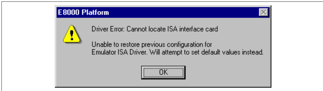
Figure 2.11 PC Interface Board Connection Error Message Box
