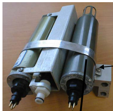
Slide sensor(s) out of bracket
