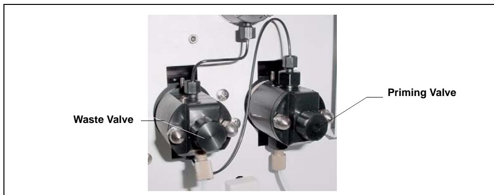
Figure 4-2. Waste and Priming Valves
