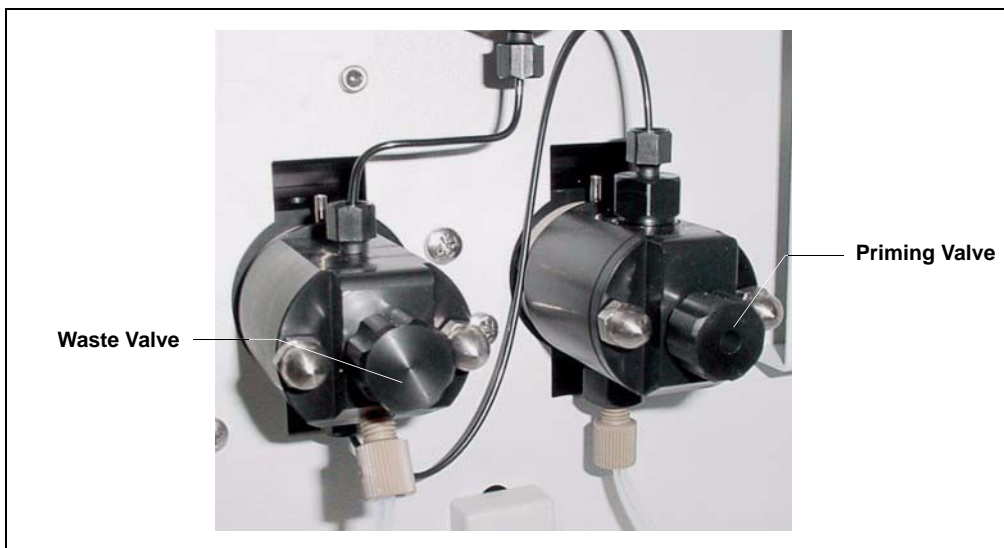
Figure 5-7. Waste and Priming Valves
