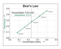
unknown concentration is placed in the colorimeter and its absorbance measured. When the absorbance of this solution is interpolated on the Beer's law curve, as shown on the previous page, its concentration is determined on the horizontal axis. Alternatively, its concentration may be found using the slope of the Beer's law curve.
