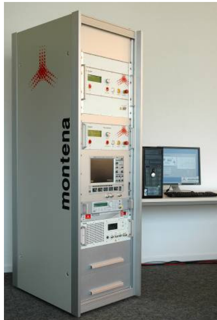
Figure 3 : Combined fully automated CS114 + CS115 + CS116 test setup
