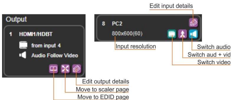
Figure 15: Switching Page – Input and Output Icons
