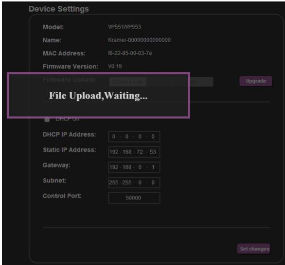
Figure 30: The Device Settings Page – Uploading the New Firmware File
