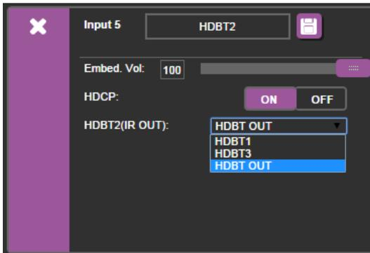
Figure 20: Switching Page – HDBT input Window
