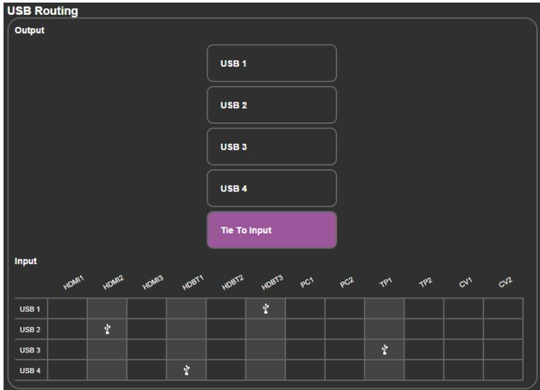
Figure 34: The USB Tied to a Selected Input
