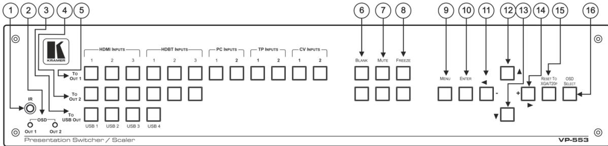
Figure 1: VP-553 Presentation Switcher/Scaler Front Panel
