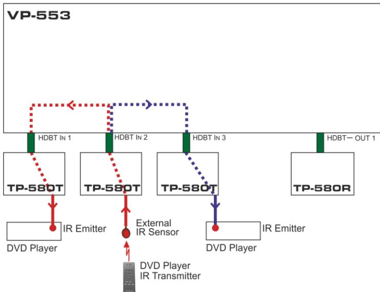
Figure 24: HDBT IR transmission Example
