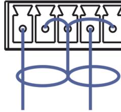
Figure 5: Unbalanced Stereo Audio Output Connection
