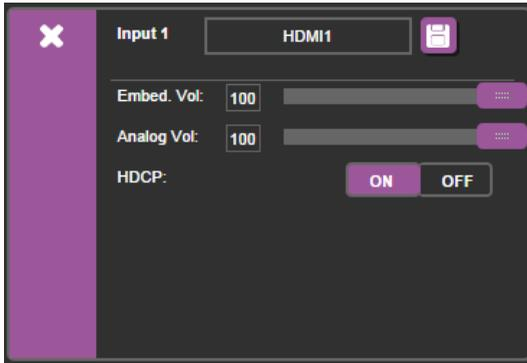
Figure 19: Switching Page – HDMI input Window
