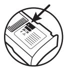
The battery pack's Active Status Indicator ("ASI") is located on the label face of the battery pack and is used to indicate battery pack status. A periodically blinking green LED indicates that the battery pack status is OK and the battery pack is ready for use. Absence of a blinking green LED indicates a battery pack problem or a depleted or missing 9V battery. Refer to the "Checking DDU-100 AED Status" section for information on battery pack LED indications.
