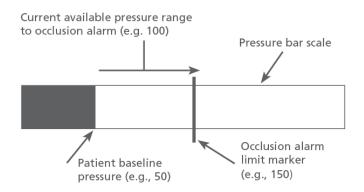
At higher limits in Selectable Pressure and in Pump mode at flow rates of 30 mL/h or more, the limit marker is placed directly in relation to the bar graph 0-525 mmHg range. For example, as shown in the figure below, in Pump mode at 50 mL/h, the limit bar will be set to 250 mmHg (about at the horizontal center); this value is relative to the left end of the pressure bar scale.
