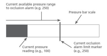
**Note:** On the device that the numeric VTBI (Volume To Be Infused) is displayed just above the Dynamic Pressure display bar for each channel. There is no relationship between the VTBI and the Dynamic Pressure display.
