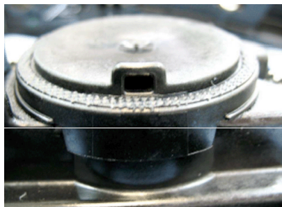
The PCV orifice is an integral part of the camshaft cover.
