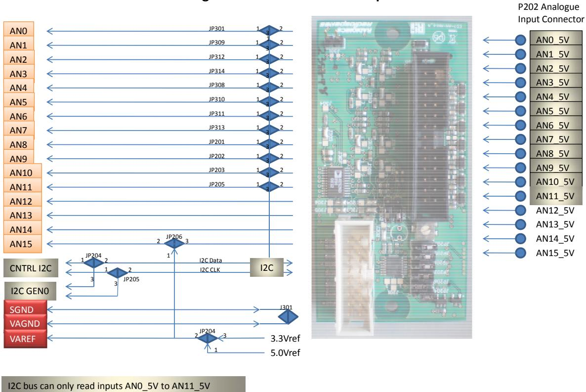
Block diagram of the Analog Module showing capability and basic link options. Normally AN0\_5V to AN15\_5V are used for the raw analog inputs. The processed analog signals are passed to the MCU via the backplane on AN0-AN15 or redirected into the on board ADC for reading via an I2C chip. With this implementation a total of 16 analog inputs are available, the first 12 of which are readable via I2C.
