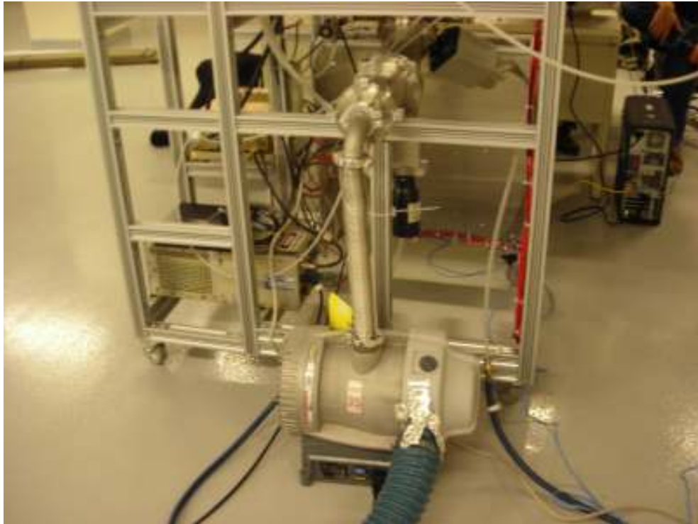
Figure 4.2. Plumbing from chamber to pump.
