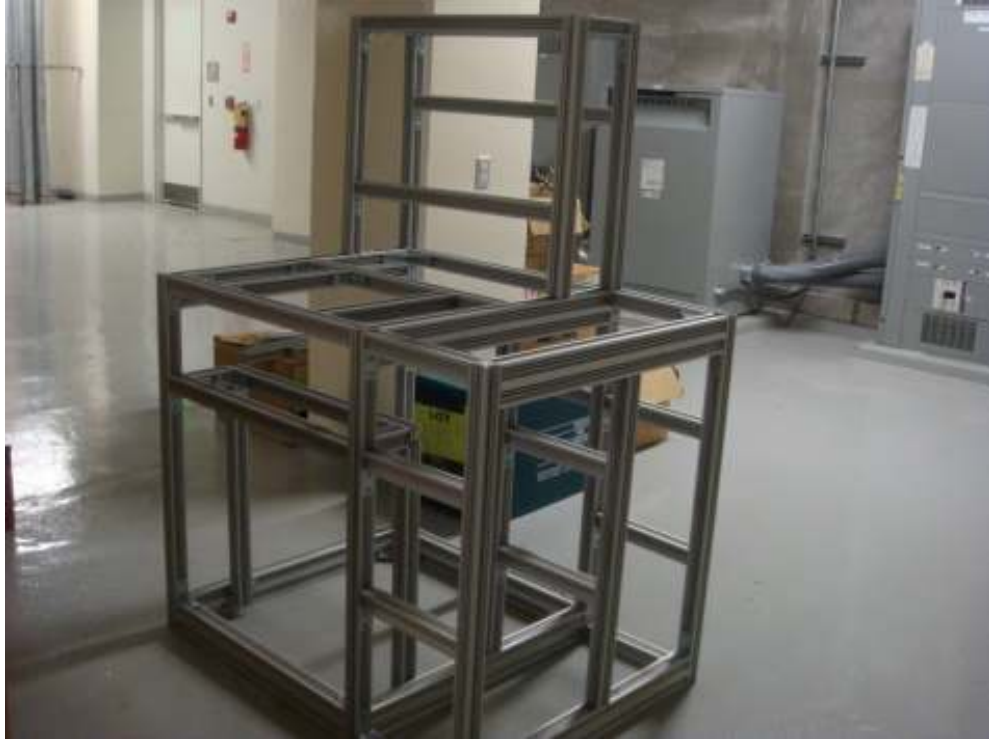
Figure 4.1. Frame used to build the PECVD machine.
