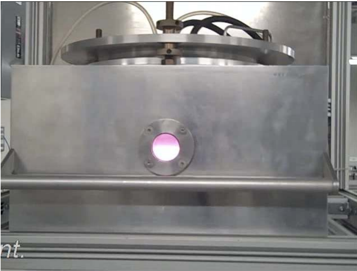
Figure 6.2. Chamber with a successful Plasma ignition.
