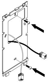
2. Connect one end of an RJ-45 cable into the wall mount connector on the Access Point as illustrated below.
