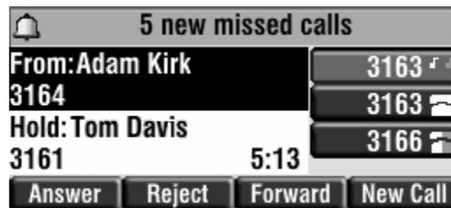
Your phone can display two call appearances at one time. If more than two calls are taking place on the same line, a counter displays on the display. Use the down arrow to access additional calls, or “appearances”.
