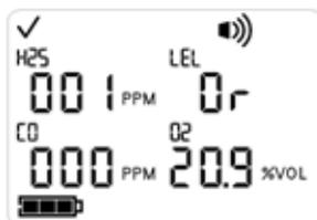
The over range alarm will normally reset itself when the gas concentration returns to a level within the sensor measuring range. However, if the LEL sensor reaches an over range condition, the alarm will latch and the instrument must be turned off and then on again to clear the over range condition.
