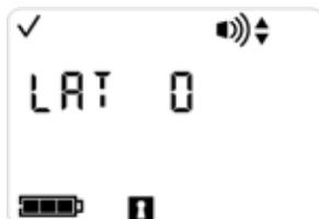
Use the Enter button to toggle between these values. A “0” value indicates “normal” alarming. A “1” indicates “latched” alarming. If the alarms are latched, to un-latch in normal reading mode, press and hold the Enter button for three seconds.
