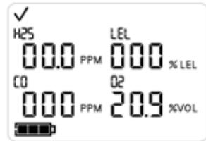
When the gas concentrations return to normal values (for example, drop below the high alarm set points or rise above the low alarm set points), and the alarm latching feature is not set, the MX4 will go back to the normal monitoring screen.
