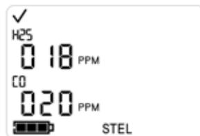
The STEL (Short Term Exposure Limit) for the toxic sensors is reset every time the unit is powered down. In addition, pressing the Enter button resets the TWA values. The STEL readings are calculated as a running average of readings over the last 15 minutes.
