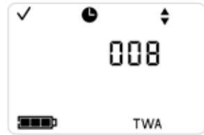
The TWA time base is a time (in hours) that is used in calculating the TWA values. The default value is 8 hours. Valid values for the TWA interval are from 1 to 40 hours.
