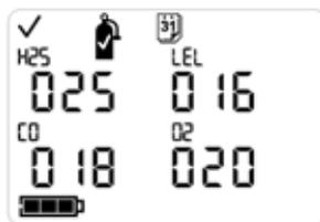
Pressing the On/Off/Mode button from the Days Since Calibration screen displays the Bump Test screen (if enabled in the configuration mode).
