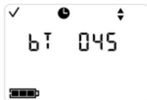
This value may be selected in 5 second intervals from 30 seconds to 300 seconds. The bump test period will end when the selected timeout value is reached regardless of whether the test has passed or failed.
