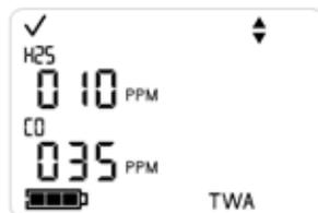
If changes are desired, press the Enter button. The first TWA alarm value flashes. To adjust this value, use the Enter button. Once the desired value is met, press the On/Off/Mode button to select the next TWA alarm value.
