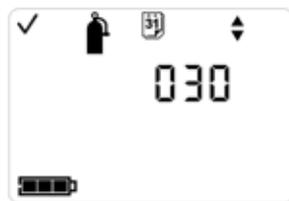
If no changes are needed, press the On/Off/Mode button to move to the next screen (the Clock Setting screen).
