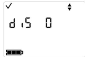
Use the Enter button to toggle between these values. After the desired display mode setting is selected, press the On/Off/Mode button to display the Confidence Indicator screen.
