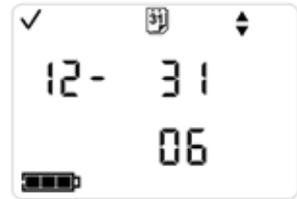
If changes are desired, press the Enter button. The first value to flash is the numerical month setting. To adjust this value, use the Enter button. Once the desired value is met, press the On/Off/Mode button to submit the value and move to the day value.
