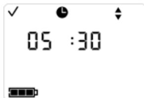
If changes are desired, press the Enter button. The first value to flash is the hours setting of the clock. To adjust this value, use the Enter button. Once the desired value is met, press the On/Off/Mode button to submit the value and move to the minute value.
