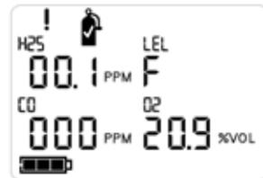
A full span value greater than 70% of the applied calibration gas value indicates a healthy sensor. A full span value between 50% and 70% of the applied gas concentration are considered to have marginal sensitivity and limited life remaining. Sensors will fail calibration if the full span value is less than 50% of the applied calibration gas concentration. If a sensor fails calibration, the display reading for that sensor will be replaced by the letter
