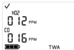
Pressing the Enter button resets the TWA values. The time base for TWA calculation may be set in the configuration mode. The default time base is set for 8 hours.
