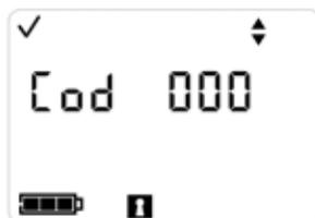
If no changes are needed, press the On/Off/Mode button to return to the Zero screen.
