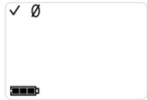
Pressing the On/Off/Mode button from the Zero screen displays the Peak Readings screen.
