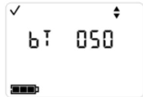
Use the Enter button to increment the display to the desired value. After the desired setting is selected, press the On/Off/Mode button to display the Bump Test Timeout screen
