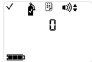
After the desired setting is selected, press the On/Off/Mode button to display the Cal Due Setpoint screen.
