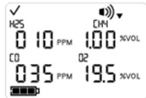
If changes are desired, press the Enter button. The first low alarm value flashes. To adjust this value, use the Enter button. Once the desired value is met, press the On/Off/Mode button to submit the value and select the next low alarm value. Continue this process until all four low alarm set points have been set.
