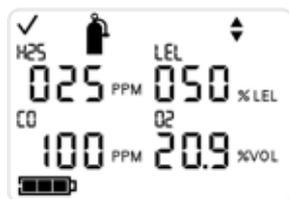
If changes are desired, press the Enter button to begin editing values. The first Cal Gas Set Point value flashes. To adjust this value, use the Enter button. Once the desired value is met, press the On/Off/Mode button to select the next Cal Gas Set Point value.
