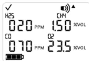
If changes are desired, press the Enter button. The first high alarm value flashes. To adjust this value, use the Enter button. Once the desired value is met, press the On/Off/Mode button to select the next high alarm set. Continue this process until all four high alarm set points have been set.
