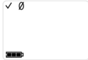
When the zeroing process is completed, calibration can be initiated by pressing the On/Off/Mode button. The instrument display will flash the calibration gas concentration for the first sensor to be calibrated. The calibration cup should be attached to the instrument and the calibration gas applied at a flow rate of 0.5 liters per minute.
