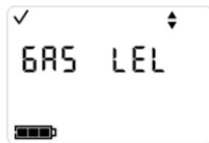
From this screen you set the combustible gas mode by toggling between the two options – lower explosive limit (LEL) or methane (CH<sub>4</sub>). Use the Enter button to toggle between these values. After the desired combustible gas operating mode selected, press the On/Off/Mode button to display the zero initiate screen. If the mode is changed, the sensor will be automatically put into the calibration fail mode to ensure correct calibration.
