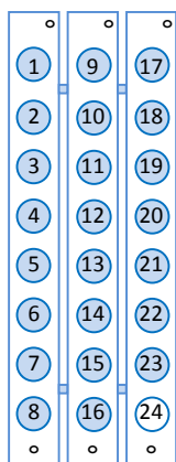
Figure 3. Positions of the 23 qPCR master mixes in each block of 3 x 8 tubes. Tube number 24 is empty and can be used for orientation of the 24 tube block. The hole in the upper right corner of each 8-tube strip (depicted as °) marks the beginning of the strip and the centered hole marks the end of the strip. The tube numbering refers to the tube numbering in the Interpretation table.
