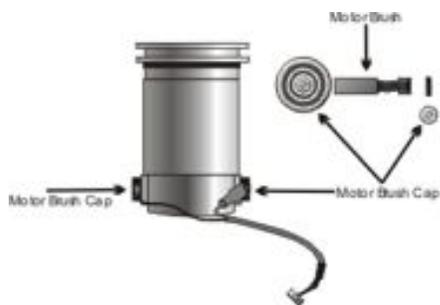
Use a flat blade screwdriver to loosen the motor brush cap. Inspect the motor brush for length. If the length is under 1/8 inch (3 mm), the motor brush needs to be replaced. If the motor brush is over 1/8 inch (3 mm), put the existing brush back into the motor and replace the motor brush cap.
