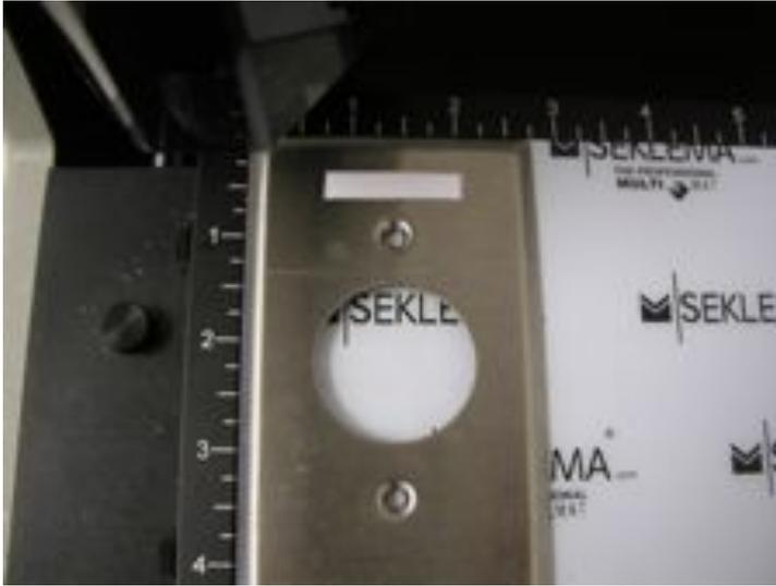
Move the spindle using the X, Y and Z buttons on the engraver, so that the tip of the cutter is directly over the upper left hand corner of the engraving area. The pictures below show the spindle/cutter tip correctly positioned in the upper left corner of the engraving area.
