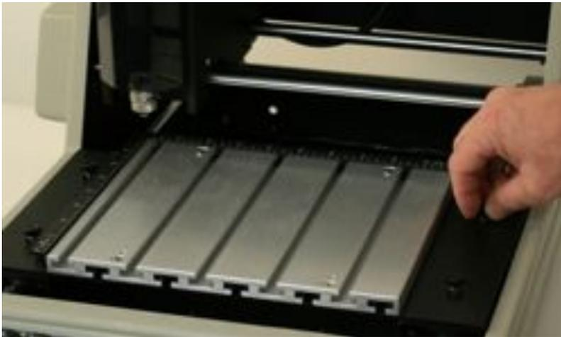
Remove the T-Slot table.
