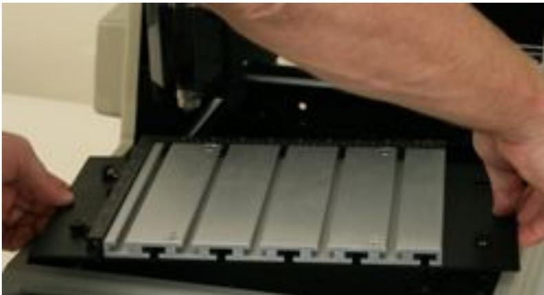
Install the vise and secure it by tightening the 4 mounting screws. Make sure the 4 vise pins are installed on the top of the vise.
