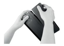
2. Remove the internal cover of enclosure and insert the hard drive horizontally inside the enclosure, connecting the connector SATA of hard drive with that of the enclosure, push the hard drive firmly until fitting it well with enclosure.
