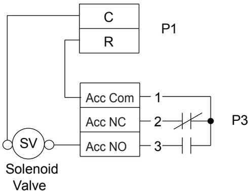
**Figure 9b: Open Loop Solenoid Valve Connection Option**
