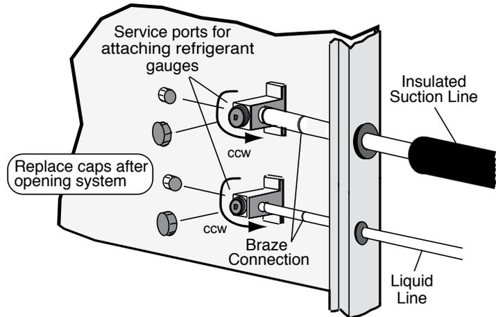
Figure 14: Attaching the Air Coil
