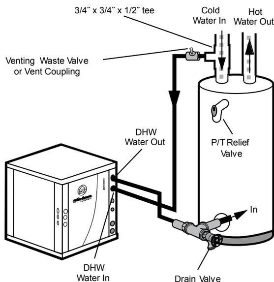
**Figure 11: Desuperheater Installation in Preheat Tank**
