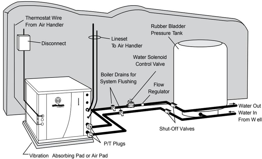
**Figure 5: Open Loop Solenoid Valve Connection Option**
