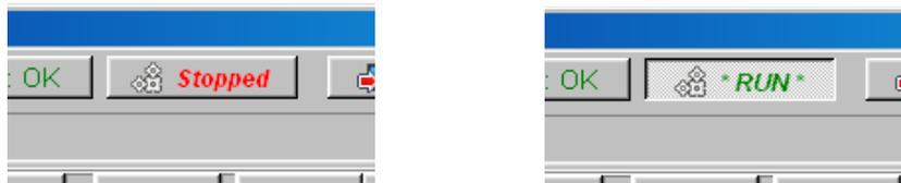
When the cycle starts to run from stopped state, all the internal parameters (flags, options, inputs thresholds...) are set to their default.
