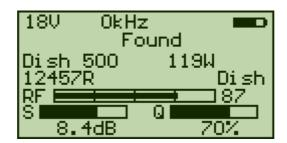
Once the correct satellite is found, then the dish can be "peaked" using the SNR bar and the quality bar for reference. The SNR should be as high as possible, and the Quality measurement should be as high as possible. If the beeper is enabled, when a signal is locked, the pitch of the signal is reporting the SNR.
