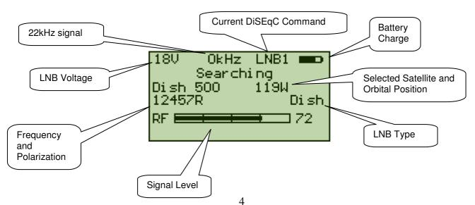
The signal level will increase on the signal bar if any satellite signal is detected. If the beeper is enabled, then the pitch of the beeper will increase with signal strength. Once the instrument locks on a satellite transponder, the display is changed. Once locked on a transponder, the SNR (signal to noise ratio) bar and the Quality bar (derived from BER - bit error rate) are displayed.
