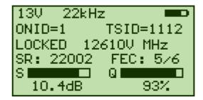
As each frequency is checked, the RF value is shown. When a DVB-S signal has locked, the display changes to show the Symbol Rate and FEC. When the NIT information is available, it is also shown. (ONID is "Original Network ID", and TSID is "Transport Stream ID")
