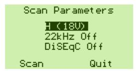
This function searches for a DVB-S signal every 10Mhz. It starts at the lowest frequency for the LNB type (10670MHz for Universal) and samples every 10MHz until a signal is detected. The "**UP"/"DOWN**" buttons select the direction of the search.
