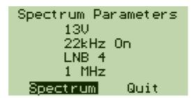
The "Up" and "Down" buttons select the settings of the LNB Voltage, 22kHz signal, and DiSEqC, and the Spectrum bandwidth and the "OK" button changes the setting. Pressing "OK" when "Spectrum" is highlighted will display the spectrum.
