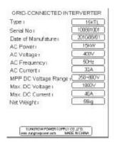
Fig 3-1 Nameplate of Inverter
