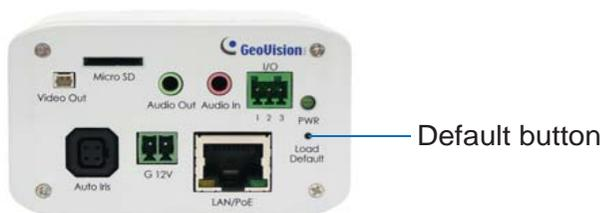
3. Plug the power cable, or the network cable to power on the camera through the PoE adapter. The status LED on the front panel of the camera turns on and then off twice. This may take about 30 seconds.
