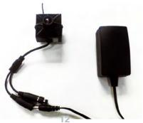
3. Plug the receiver power supply (5VDC, 1.5A) to the receiver's DC IN port and the other end to an electrical power outlet. Next, connect the AV cable out from the receiver to your TV/monitor or recording devices (VCR or DVR) AV input.
