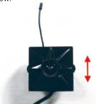
2. Connect the power adapter plug into the power socket attached to the camera and then connect the power adapter (5VDC, 1.5A) into an electrical power outlet as shown below.
