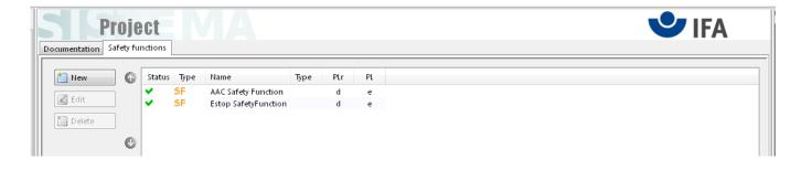
This safety system includes two safety functions: single-beam area access control sensor safety function and an E-stop safety function.
