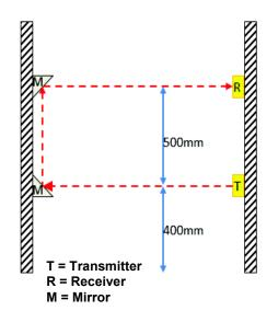
With reference to the EN ISO 13855: 2010, Appendix E standard, for two-beam applications, the two mounting heights are 400 mm and 900 mm from the ground or panel level that correspond to adequate risk reduction and application practice.
