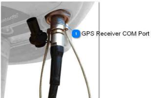
One end of the Power cord is connected to the GNSS receiver and the other end to the SETTOP battery.
