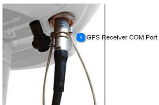
One end of the Power cord is connected to the *Radio Link Port* of the SETTOP Radio-Link device and the other end is connected to the GNSS receiver
