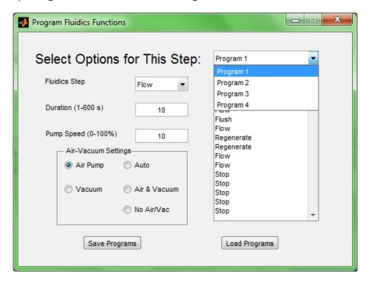
Use the "Program" menu to select which program you will use for cortisol detection. This is stored on the instrument and the instrument is limited to four different program sequences. For the cortisol assay Programs 1 and 2 will be set up.
