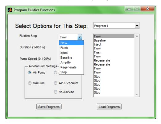
Select the step type in the dropdown menu. These steps will equilibrate the sensors prior to injection, zero the sensor signal, set the valves for injection, flow the sample over the sensor surface, flush the
