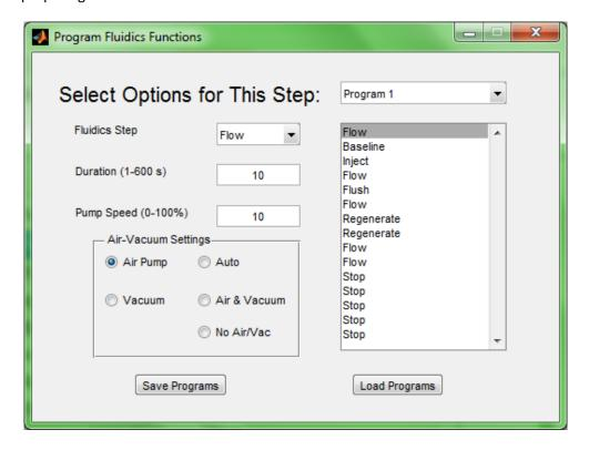
Use the "Duration" and "Pump Speed" boxes to select the appropriate values for these. Use the "Air-Vacuum" Settings to select whether the air pump is turned on or off. This pressurizes the buffer chamber to prevent air bubbles from forming. This will be used for "System Preparation and Cleaning".
