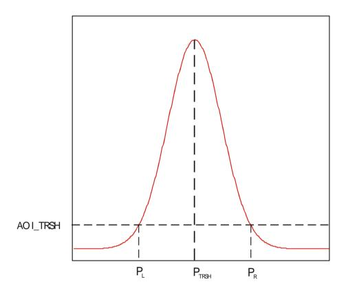
The position value of the laser line is approximated:  $P_{TRSH} = (P_L + P_R) / 2$ . In order to simplify the digital representation the division over 2 is not performed and thus an integer representation with one subpixel is realised. The evaluation of 1728 rows delivers a position range from 0 to 2047 pixels (12 bit).
