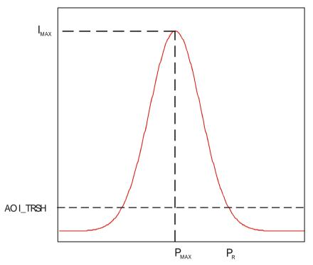
The calculation of position value is performed with simple pixel accuracy, i.e. the evaluation of 1728 rows delivers a position range from 0 to 1727 pixels (11 bit). If there is more than one local maximum, the position of the first maximum (starting from row zero) is used.
