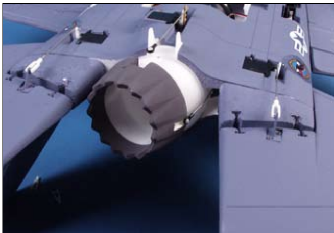
Thrust nozzle shown with right thrust mixing activated.
