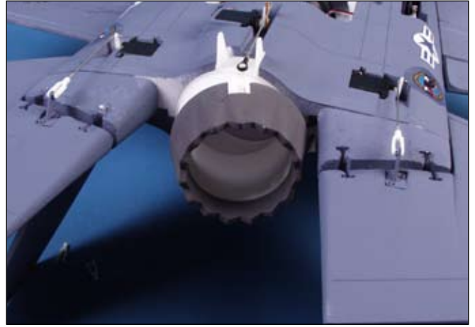
Thrust nozzle shown with up thrust mixing activated.
