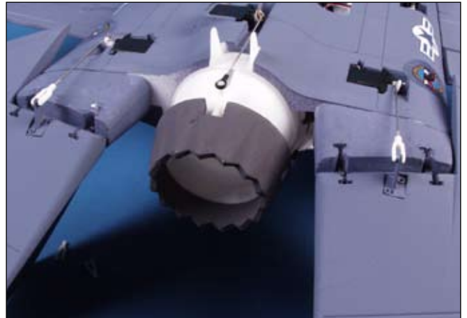
Thrust nozzle shown with down thrust mixing activated.
