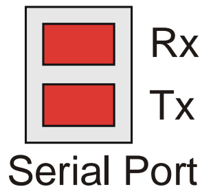
Figure 6.10 – Automation Equipment Port Receive & Transmit LEDs The LED's flash when the HENX2XXTXXX is communicating.
