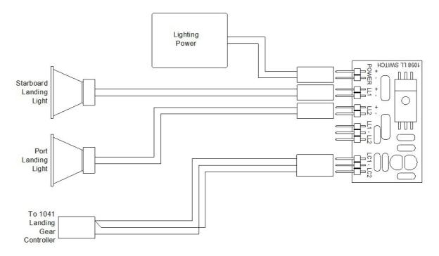
Connecting to 1070 series Landing Gear Controller
