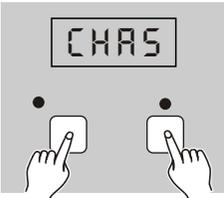
2. Keep pressing AUDIO/DEL button, tap the button that holds the chase you wish to delete, all LED's shall flash briefly three times indicating this chase has been deleted.
