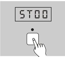
1. Apply power on, tap Chase button causing its LED to light or flash, the Segment Display shows "ST00".
