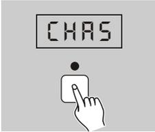
2. Press and hold down Record button for 3 seconds, the Record LED will flash indicating recording is active, the Segment Display reads "CHAS", and the recorded chases will be indicated by the lit LED's near 1-40 buttons.
