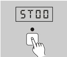
3. Tap one of 1-40 buttons to select a chase, its LED I flashes, the Segment Display shows "ST00" or "ST01".
