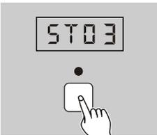
1. When the chase or memory is playing, you may tap AUDIO/DEL button, its LED is lit, which refers to that Audio mode is active, the chase or memory shall be subject to the audio signal detected by built-in Mic.
