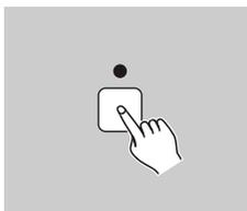
4. Tap AUDIO/DEL button, all LED's shall flash briefly three times indicating the step has been deleted.
