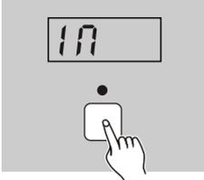
3. Press Scene button to receive record data, the Segment Display shall show "IN" indicating this unit is receiving file data. Any button doesn't work until the Segment Display shows "End".
