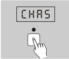
2. Press and hold down Record button for 3 seconds, the Record LED's will flash indicating recording is active, the Segment Display reads "CHAS", and the recorded Memories will be indicated by the lit LED's near them.
