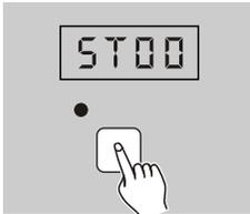
3. Tap the button(Memory 1-8) you wish causing its LED to flash, the Segment Display shows "ST00" or "ST01".
