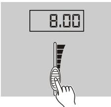
4. Move Fade time slider to adjust fade time for the current step from instant to 10 minutes, the Segment Display shows the fade time.,
