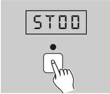
1. Apply power on, tap Chase button causing its LED to light or flash, the Segment Display shows "ST00".
