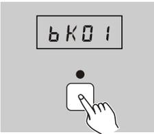
1. Apply power on, tap Scene button causing its LED to light or flash.
