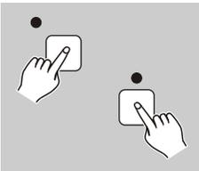
5. Keep pressing Record button, tap any of 1-40 buttons to record the scene into this button, all LED's will flash 3 times briefly indicating this operation.
