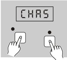
2. Keep pressing AUDIO/DEL button, tap the button that holds the Memory you wish to delete, all LED's shall flash briefly three times indicating the Memory has been deleted.
