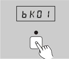
1. Apply power on, the Segment Display reads "bk01", tap Scene button causing its LED to light or flash.
