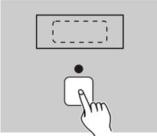
3. Before you can receive record data, be sure the second unit is in "RECEIVE" mode. Press Scene button to send record data. Now, any buttons doesn't work until the Segment Display shows "End".
