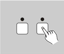
3. Press and hold down Record button for 3 seconds, both Scene and Record LED's will flash indicating recording is active, and the recorded scenes will be indicated by the lit LED's.
