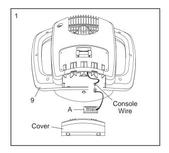
Remove the paper from one side of the adhesive pad, and press the pad onto the back of the receiver (A). Then, remove the paper from the other side of the adhesive pad and press the receiver onto the interior wall of the Console (9) in the indicated location.
