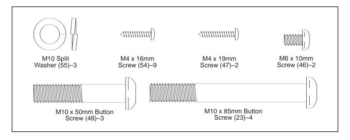
1. While another person lifts the front of the Frame (1), attach the Front Stabilizer (2) to the Frame with two M10 x 85mm Button Screws (23).
