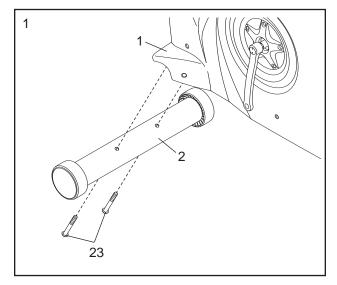
2. While another person lifts the rear of the Frame (1), attach the Rear Stabilizer (3) to the Frame with two M10 x 85mm Button Screws (23).
