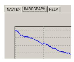
The second tab contains the BAROGRAPH. The measuring data are represented in the diagram from left to right. I.e. the current measured value is on the right side of the curve. The barograph has a measuring interval of one minute and a resolution of 0,1hPa.
