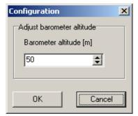
The air pressure sensor in the WIB2B measures the absolute air pressure. Because air pressure is normaly referred to sea level, a too small measurement value is displayed without correction, if the device is above sea level.
