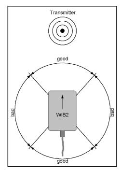
The internal ferrite rod antenna of the WIB2B has a directionality. For good reception the equipment must be operating flat lying.
