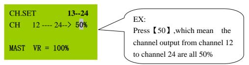
STEP 7: Press 【ENTER】 to output and the LCD will advance to the next channel to be set.
