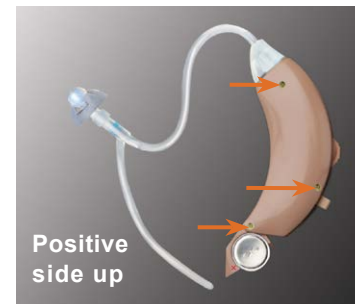
Screws on Hearing Aid Body
