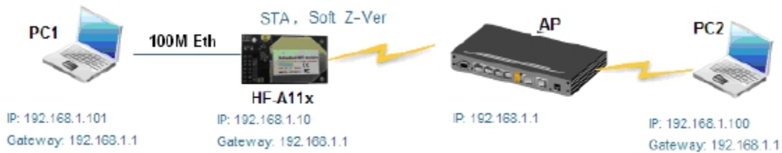
Figure 20. WIFI232-A11 Ethernet Interface Networking (As STA, Z-Ver)
