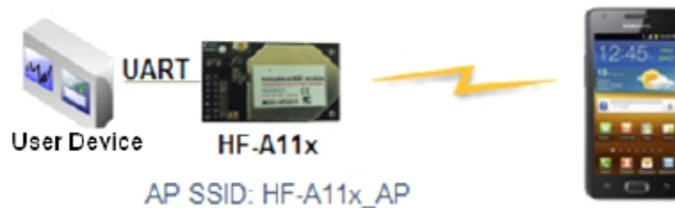
Figure 32. Wireless Control Application
